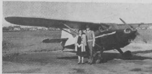
Mr. and Mrs. Smith and the Stinson VOYAGER which they are taking to Indo-China. It has a 150 H.P. 6 cylinder engine, can carry 4 passengers and 130 lbs. of luggage, cruising speed of 125 miles per hr. with a range of 500 miles. Takeoff and landing can be accomplished in less than 100 yards—altogether a practical plane for mission work.
